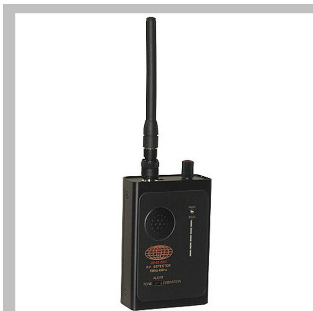
Fig.26 – MACE-JM20pro (RF Detector)
